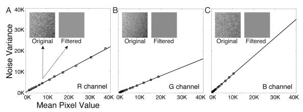
**Figure 6.** Characterizing sensor noise for a CMOS sensor. Noise variance is plotted as a function of the 16-bit mean pixel value in thousands for the **A** red color channel, **B** green color channel, and **C** blue color channel. Each symbol represents a different image with a different exposure. The line shows the fitted noise model (Equation 3). Best-fit parameter values are in the main text.
