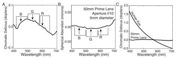
**Figure 3**. Chromatic aberrations in a 50mm prime lens. A Change in chromatic defocus with wavelength. Arrows mark the peak sensitivity of each color channel. Brackets indicate the width at half-height of each color channel's wavelength sensitivity function (see Section 2.3 & Fig. 5). B Change in spherical aberration with wavelength. C Comparison of chromatic defocus in a 50mm prime lens (same as in A) with chromatic defocus in the human lens.
