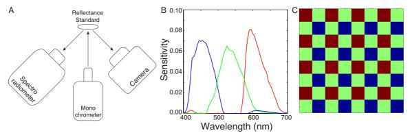
Figure 5. Characterizing the sensor array. A The physical setup used to measure the wavelength sensitivity of each color channel. B Estimated red, green, and blue pixel wavelength sensitivity functions. C Spatial sampling pattern of the Bayer color filter array.
